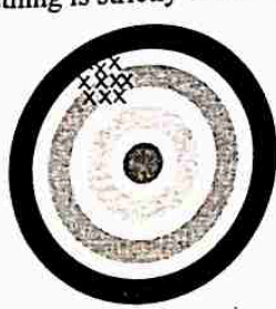
Precision Points are close to one another but not near the center.
